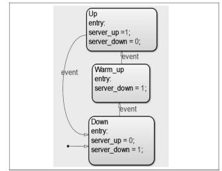
Fig. 9: State diagram for Attack(Warm-Up)
