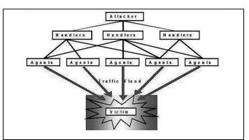
Fig. 1: Components of a DDoS Attack
